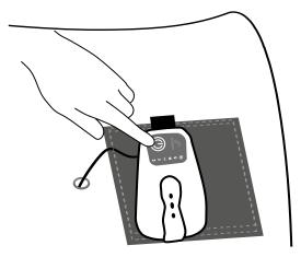
Turn the EQUIMETRE off by pressing the button during 3 secondes. All LEDs should turn off.
